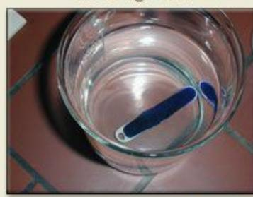
The still hot glassy product is being pulverised by immersion into cold water
