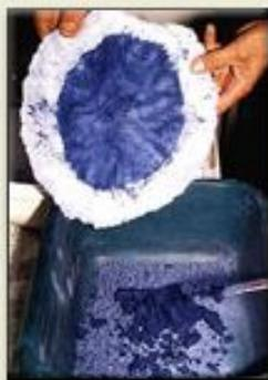
The resulting mass is kneaded with wax and water and pressed through fine cloth. The less valuable coarse "ultramarine ash" stays in the cloth
