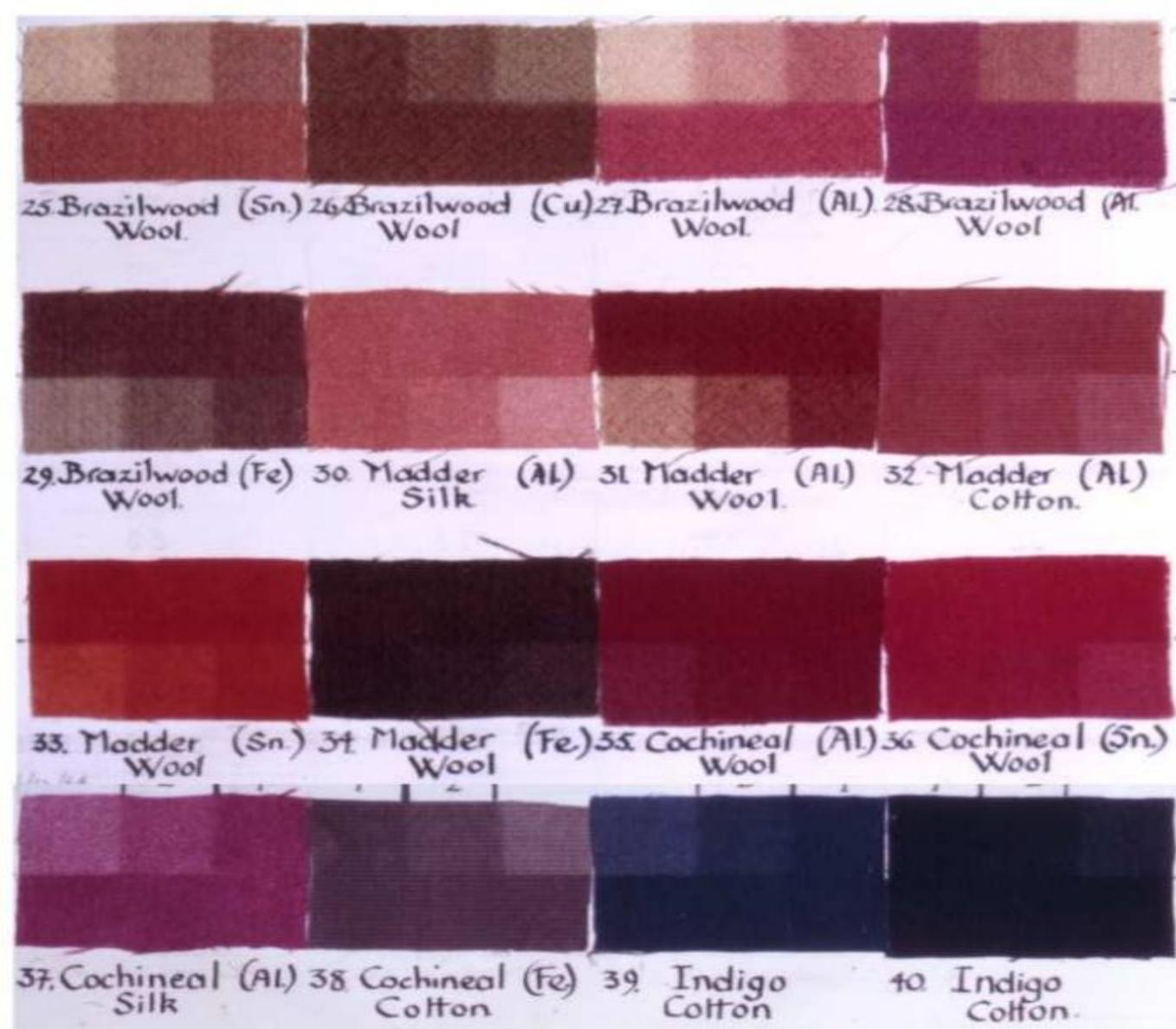
Light fastness tests of textiles dyed with natural colorants. Small squares of each sample were exposed to light of varying intensities and for different durations. The squares exposed to the brightest light for the longest time have faded the most.
